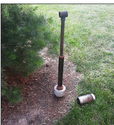
Figure 1 An example of a slide hammer device that is used to collect samples used to measure soil bulk density. Courtesy: Hans Klopp
