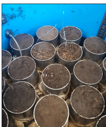
Figure 2 An example of samples that were collected to measure bulk density that were trimmed to be flush with the metal rings used to collect the sample.
